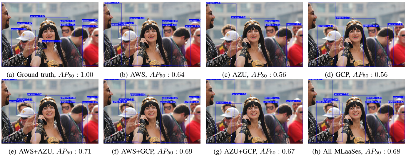
Fig. 2: Visualization of the predictions of object detection services. We display the ensemble predictions and the corresponding metrics under different MLaaS combinations.
